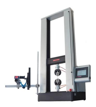
USED TO CONDUCT HIGH-PRECISION MEASUREMENT OF EXTENSION
